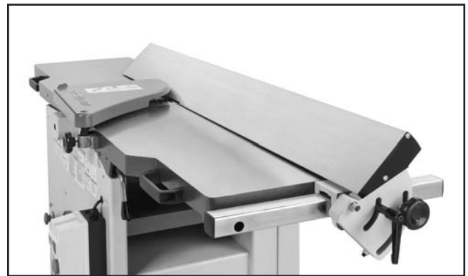
Figure 6. Fence at 45° outward position.
